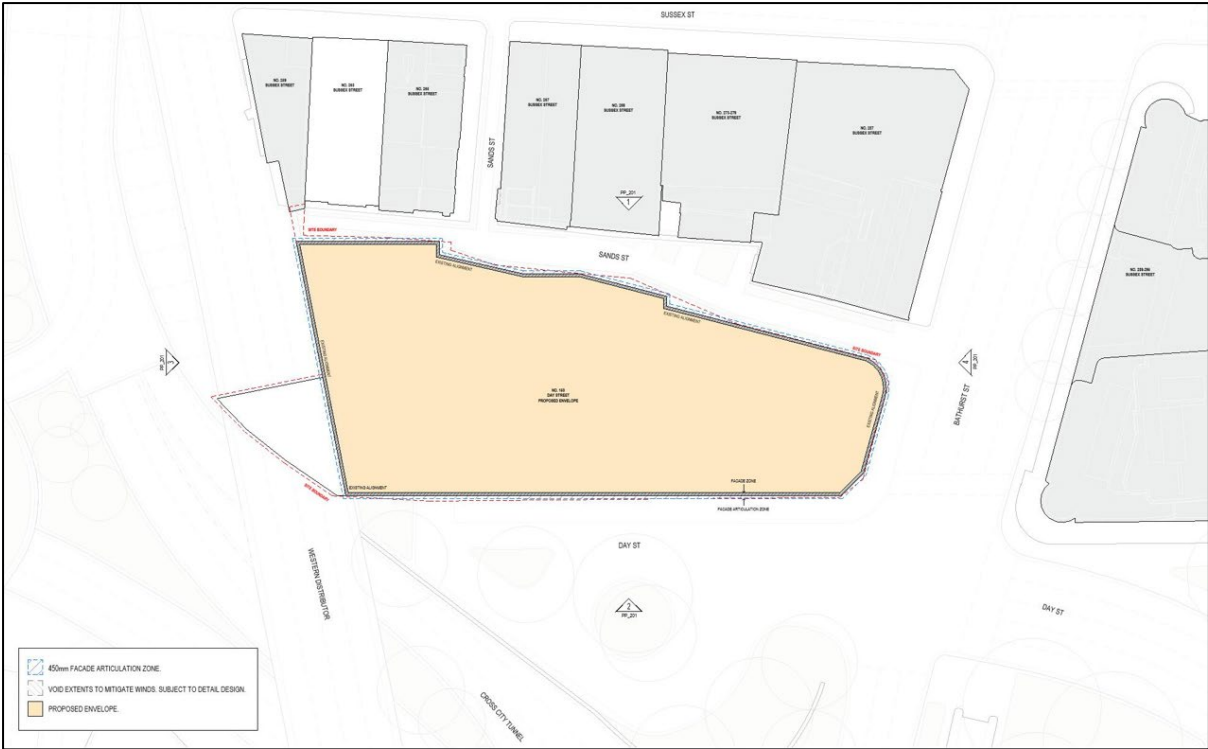
Figure 3 – Building Envelope – Level 02
